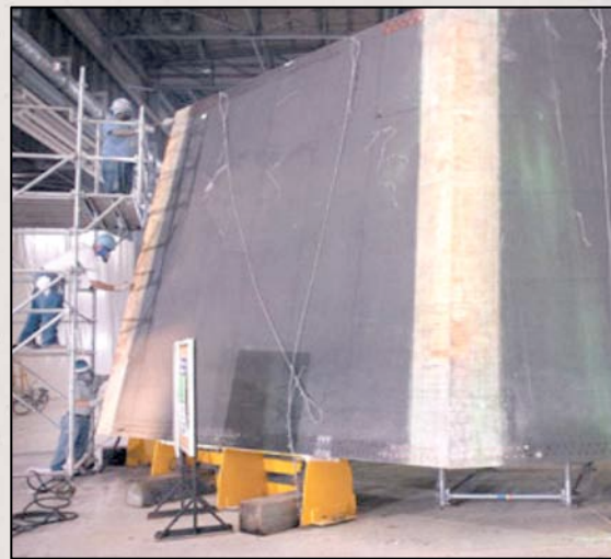
Shipbuilders at Gulfport's Composite Center of Excellence putting the finishing touches on an AEMS mast for an LPD 17 class ship
